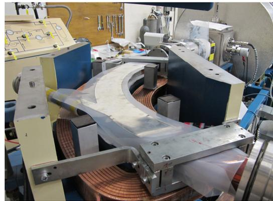
**Fig. 2:** Installation of the new LE magnet coils (top yoke removed).
