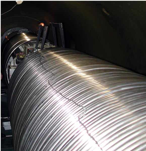
**Fig. 1:** View of the inside the EN TANDEM accelerator. For maintenance work the terminal shell has been taken off and the potential rings have been moved aside in order to make room for the cleaning of the column.
