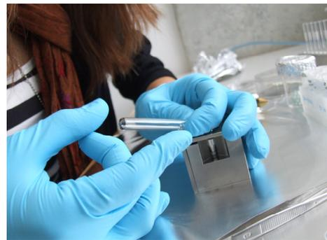
**Fig. 2:** Graphite being pressed into the AMS target for measurement with MICADAS
