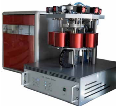
Fig. 1: The next generation automated graphitization equipment (AGE3).
