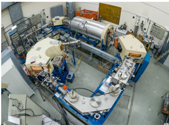
Fig. 1: The compact 0.6 MV TANDY accelerator.
