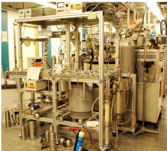
Fig. 1: The ETH in situ ^{14}\text{C} extraction system.
