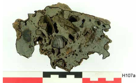
Fig. 2: Cut bloomery furnace slag with well-preserved charcoal.
