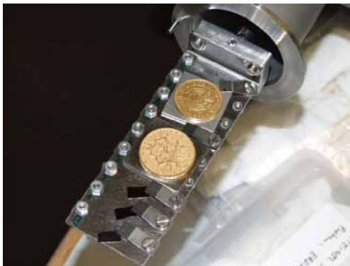
Fig. 1: One of the tasks is to identify a fake gold coin and determine the actual structure and composition of the material.
