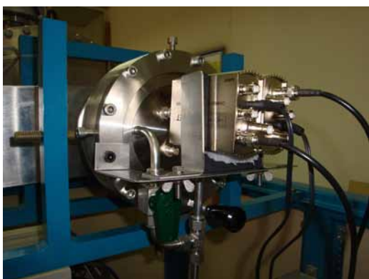
Fig. 1: The ETH \Delta E - E_{\text{res}} GIC mounted at the beam line of the 500 kV PKU AMS facility.
