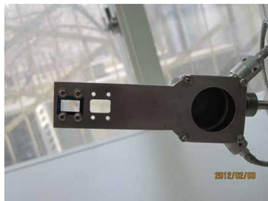
Fig. 2: Holder for the SiN degrader foils mounted on the suppressor aperture of the ^{13}\text{C} Faraday cup.
