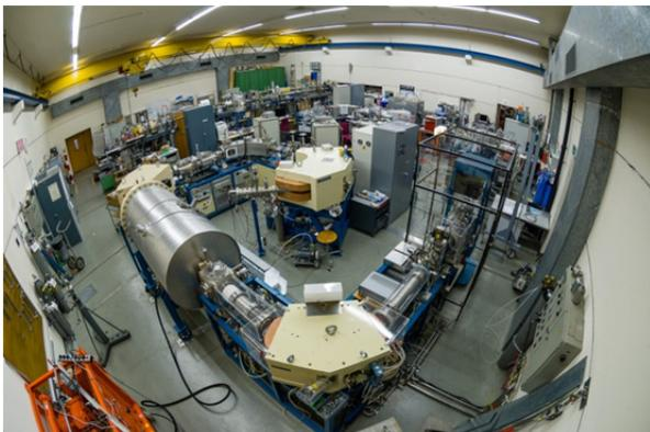
**Fig. 1:** The compact 0.6 MV TANDY accelerator.
