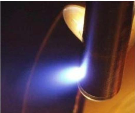
**Fig. 1:** Plasma plume at the ablation target.
