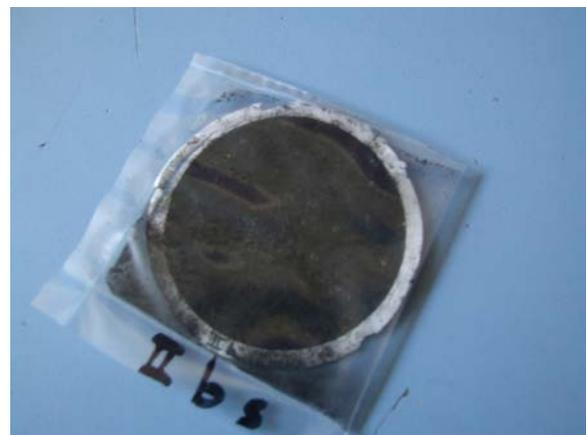
**Fig. 2:** HEPA filter used to determine airborne, particulate <sup>129</sup>I.
