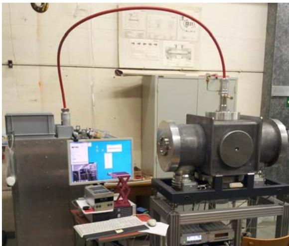
**Fig. 1:** A 300 kV power supply connected to a modified MICADAS accelerator chamber. The chamber does not contain a stripper gas system yet.
