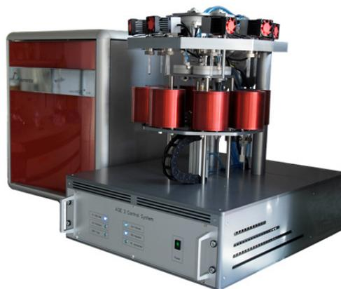
**Fig. 2:** The Automated Graphitization Equipment (AGE) is the first instrument to fully automatically combust and graphitize carbon samples.
