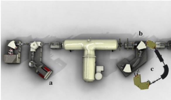
**Fig. 1:** Top view of the CEDAD AMS facility [1] with the new multi-isotope spectrometer (c).
