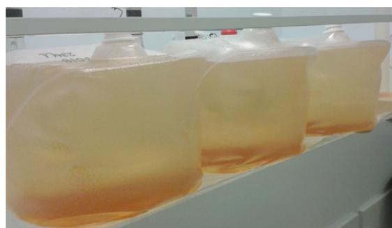
**Fig. 2:** Pre-concentration of the samples for further processing and analysis of  $^{236}\text{U}$  and Pu (iron hydroxides) and  $^{90}\text{Sr}$  (supernatant).
