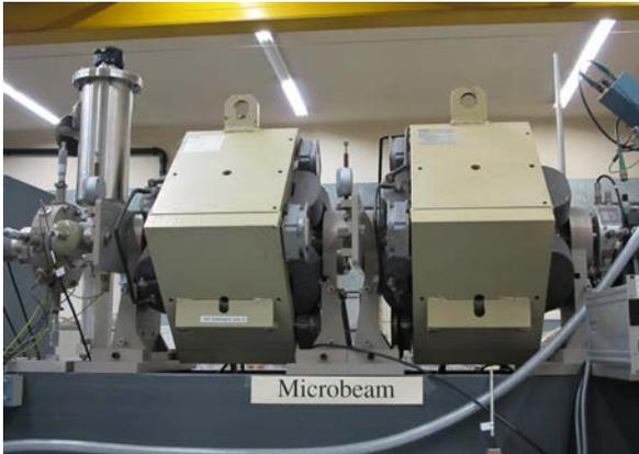
**Fig. 1:** Picture of the original micro beam setup at ETHZ, showing the quadrupole lenses.
