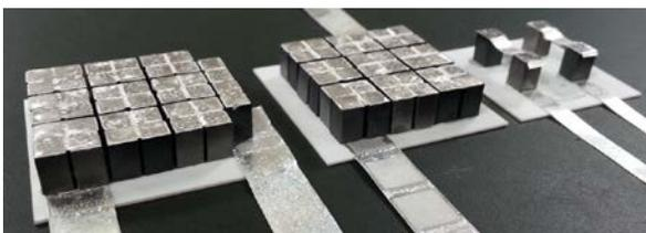
**Fig. 2:** Thermoelectric oxide converters.
