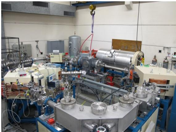
**Fig. 1:** Temporary replacement of the Pelletron system with a MICADAS-type accelerator.
