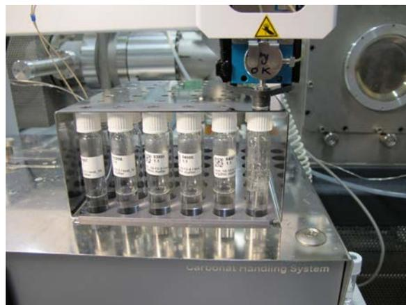
**Fig. 1:** Online  $^{14}\text{C}$  analysis of DOC samples using the WCO method.
