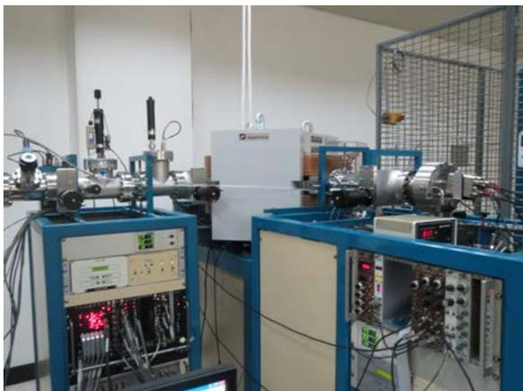
**Fig. 1:** The extended beam line including the additional 90° magnet (350 mm radius) and the ETH gas ionization chamber.
